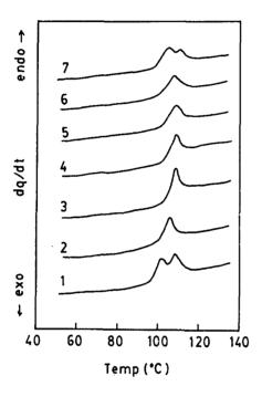
Figure 1. DSC curves of annealed PCMMA/pMSAN (50/50) blends. Wt% AN in pMSAN; (1) 7.7; (2) 13.6; (3) 21.3; (4) 26.5; (5) 32.3; (6) 39.6; (7) 45.3.
